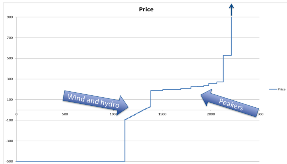
Figure 6: illustration of the aggregate simple order supply curve used for batch two of the Scripted Trials
