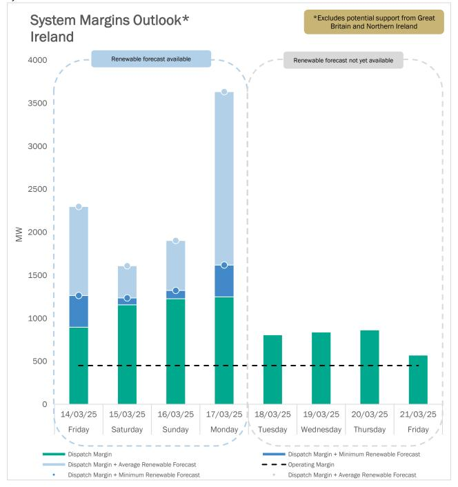
When a negative dispatch margin coincides with a low renewable generation forecast, the net renewable generation value may appear below the zero axis (low forecast: •, average forecast: •). It should be noted that the Daily Dispatch Margin and renewable generation forecast are highly variable. The outlook is based on estimates and is therefore subject to rapid changes.
